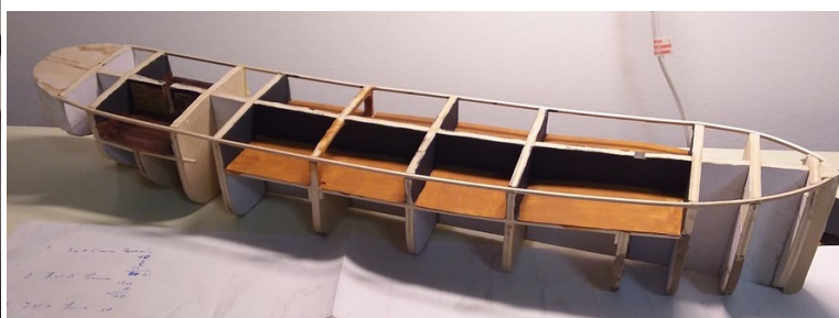
Assembling the false keel and bulkheads
