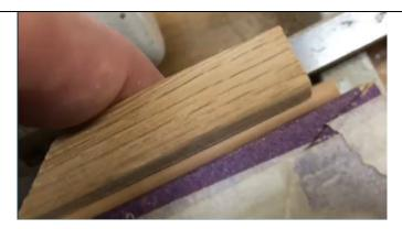
The ends of the spars are sometimes tapered 1/4 to 1/2°. He does this manually with the sanding and backup blocks running them back and forth for the partial length, stopping and checking regularly with the calipers to halt at the requisite diameter. Sometimes the ends may be rounded over. He does this with a file. Stephen finishes his parts with a brushed on coating of Watco Danish Oil, a blend of penetrating oil and varnish that dries in a matte finish.
