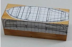
The profiles of five evenly spaced stations were marked onto the cleaned and reassembled plug. These five stations were traced from the plan onto card stock and then cut out to make templates used to check progress in rasping, filing and sanding the shape into the soft fir plug.
