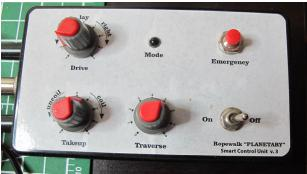
First shown was an earlier PL3.2 rope walk that can produce 2, 3 and 4 strand lines. A core is required for the 4 strand type. Sewing threads are wound on the bobbins using a sewing machine. The loaded bobbins spin opposite to the planetary assembly. The control for the ropewalk adjusts for right hand or left hand laid rope and the spool take up speed adjusts for positioning the winding point and the traverse speed for positioning the rope on the gathering spool.
