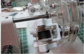
Above left we see the threads before starting when set up with the threads close at the landing point. Above right shows the back view of the loaded bobbins clamped in their cradles that will rotate them. The bobbin at the lower left of the last image is for the core or centre strand for a 4 strand rope. It feeds through the centre axle and the 4 rope strands will be wrapped around it. In the image below the ropewalk is spinning with the traverse positioning it on the spool.
