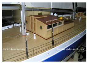
Joe's next challenges were the rigging and sails. She has wire stays with tensioning screws on the shrouds. He discovered model racing car steering turnbuckles worked perfectly and these were mounted with
