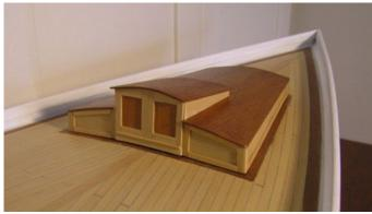
As mentioned earlier, Joe was not a fan of the supplied covering over the acrylic forward cabin (above left) so he scratch built a new one (above right). He then modified the main cabin (below). They were built in place for a snug fit using box wood and mahogany. Port holes, lights and grab rails were purchased items.
