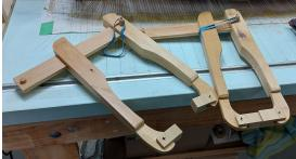
He realized that longer reaching clamps would be required to install the lower deck clamps and after a Google search he found a YouTube video on how to make "elastic band operated clamps". He made a pair of 8-1/2" reaching clamps to test them and found when set they could not be budged. So now he will be making some narrower ones to nest closer together and some much smaller clamps to be used through the gunports.
