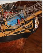
The gun rigging blocks were bought from Syren Models and the rope from Talus, a book binding supply store. He also raised the height of the roundhouses from deck level to railing level and raised the edge of the headrails with trim.
