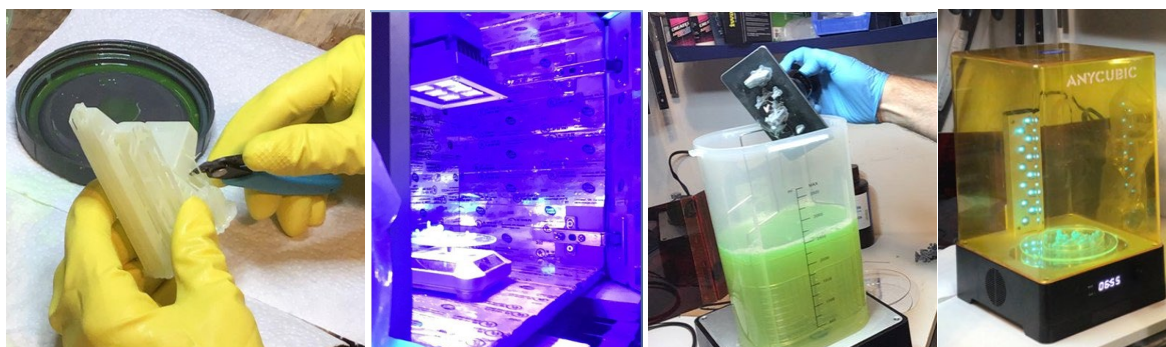
Above: trimming supports, U/V hardening, wash and cure station
