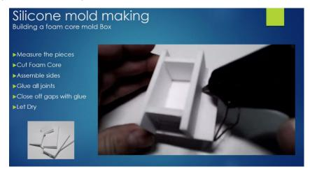
We watched a short video of the assembly of a foam core box. The material can be bought at most hobby stores, craft stores, or even Dollar Stores. The pieces are cut to size and joined together with a hot glue gun. Once the bottom and sides are joined the seams are sealed all around with hot glue. The silicone material is very watery and will seep through any open unsealed joint.
