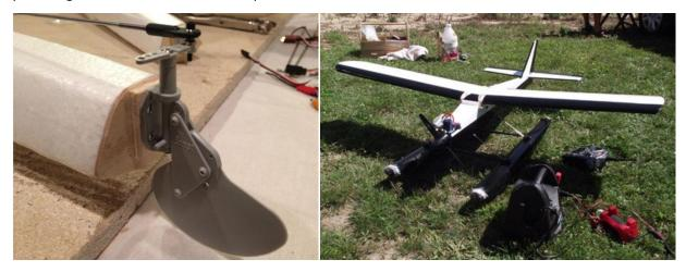
After having added weights to the nose of the floats to adjust the location of the centre of gravity he was off to the pond... and had a successful lift off and landing!
