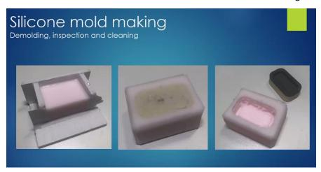
The silicone mould is then removed from the box and the part removed from the mould. Then came time to mix the resin and cast new parts.
