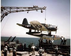
There are two types of sea planes. The first used some type of float system attached to the plane as seen above. The second being the flying boat where the airplane body is built in the shape of a boat.
