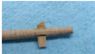
Yard Arm Stop Cleat being shaped
