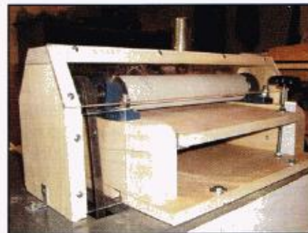
Completed sander from exit end
