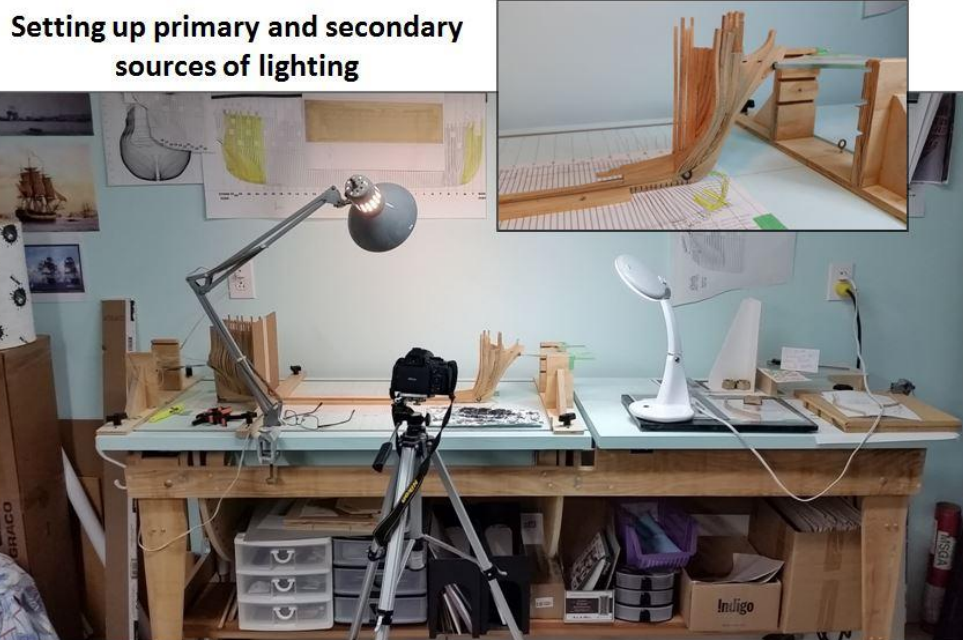
Two lamps from front sides; reflecting off table top, back wall and aluminium foil. Supplemented by one set of ceiling hung soft white florescent lights
